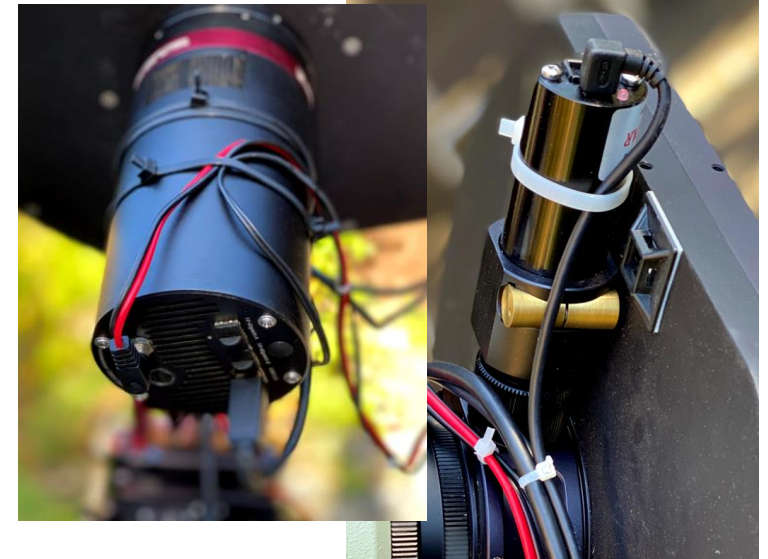
Secure the cables so no weight pulls on the power or USB port
